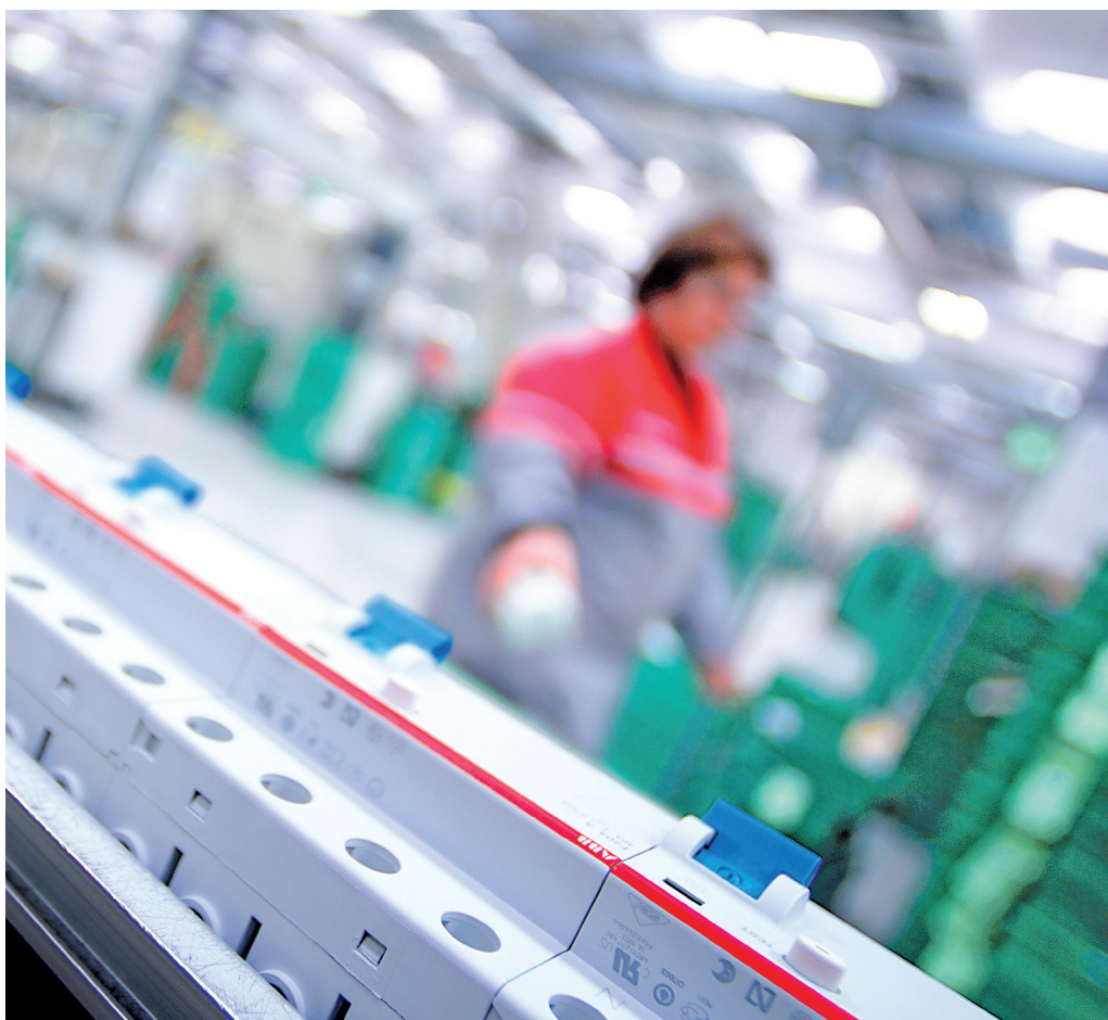
02 03 Production line of the RCCB F200 Type B
